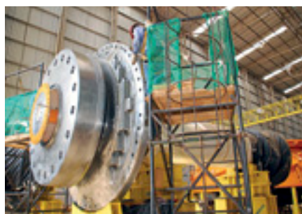
▼ Generator bearings for HPP Santo Antônio
