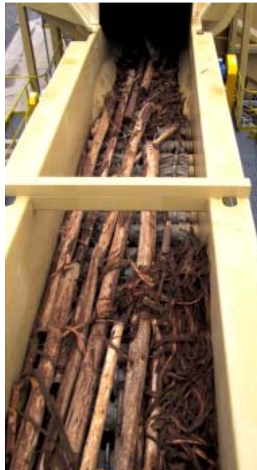
The EucaRoller™ is an Andritz innovation to remove stringy eucalyptus bark prior to the chipping operation.
