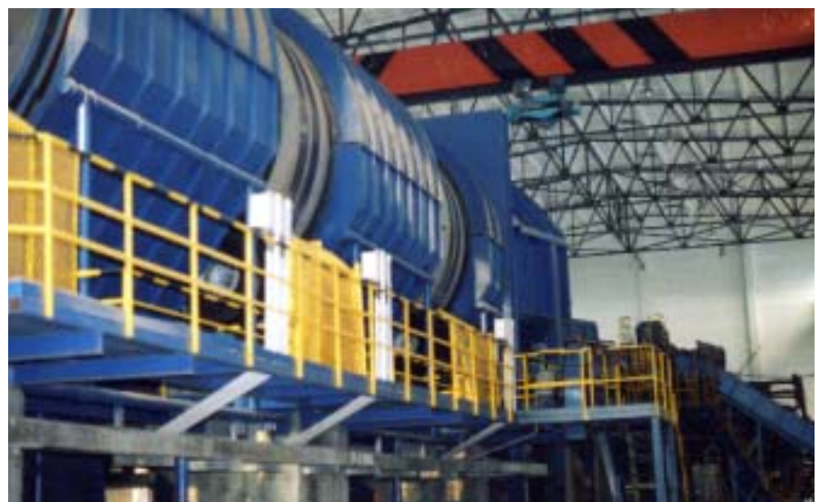
The Andritz dry debarking drum at the Yueyang Mill.
