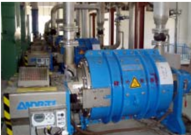
Papillon™ cylindrical refiner for the NBKP line (200 admt/d).
