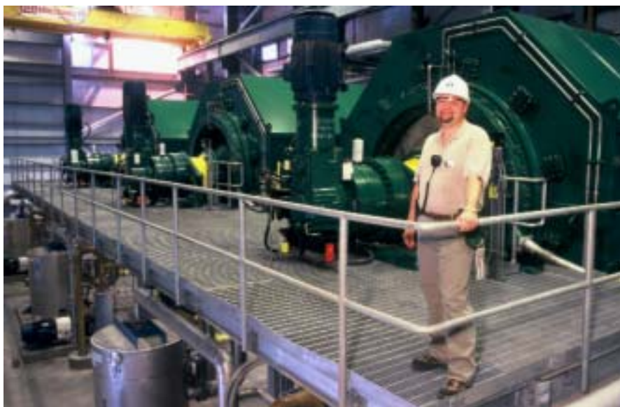
Drum Displacers at work. Danny Webb, Fiberline Operator I, in front of the Andritz interstage DD Washers in the bleach plant.
