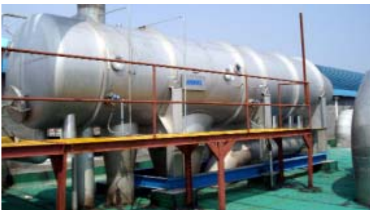
The Multi-Retention Dual Deculator® for stock deaeration on PM19.
