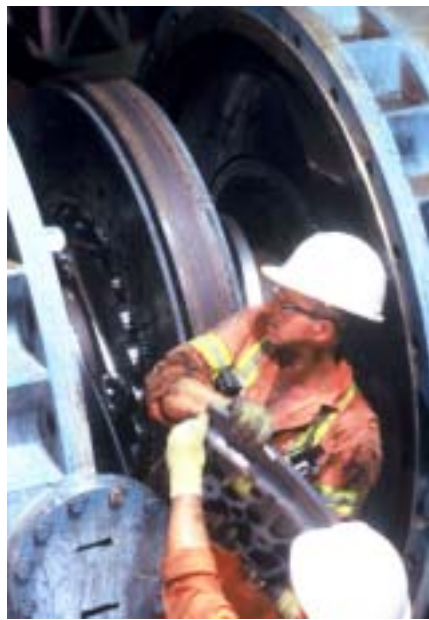
Plates make a difference. TMP Millwright Ed Westgate puts new Durametal® plates on Line #5.
