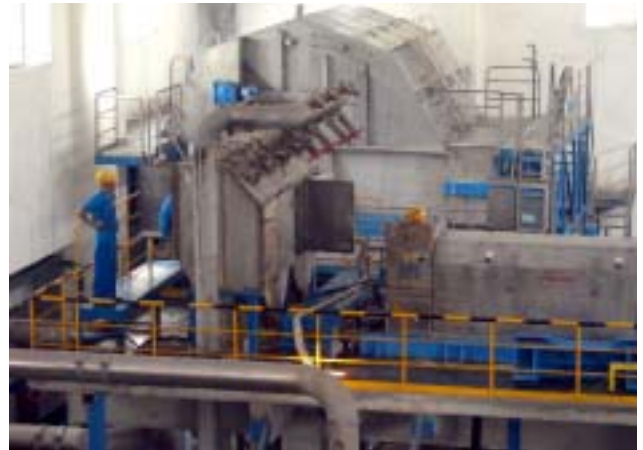
Andritz Disc Filter, MicraSieve screens, and Screw Press in operation on the P-RC APMP pulping line at Yueyang.
