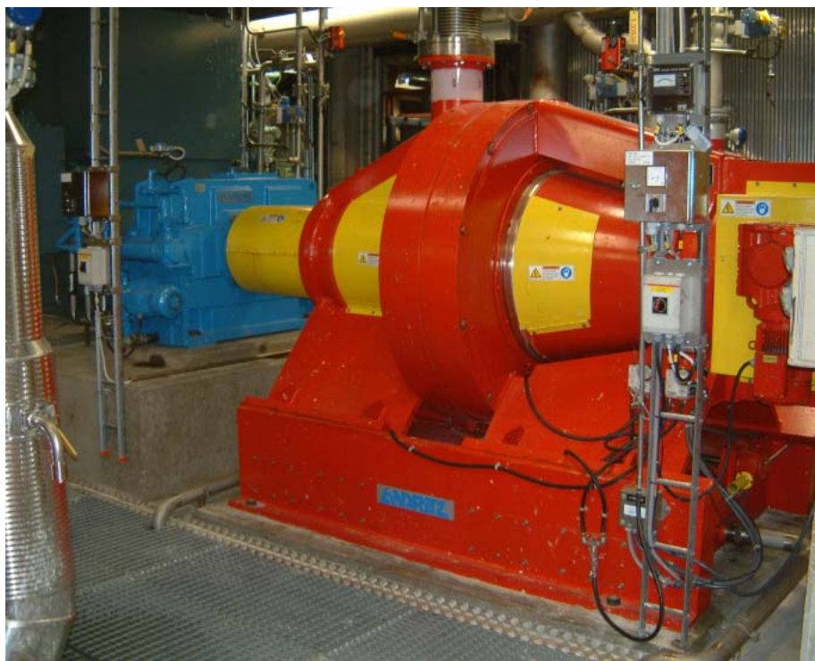
Holmen Braviken, Andritz third stage TMP low consistency Refiner — takeover in last quarter 2004.
