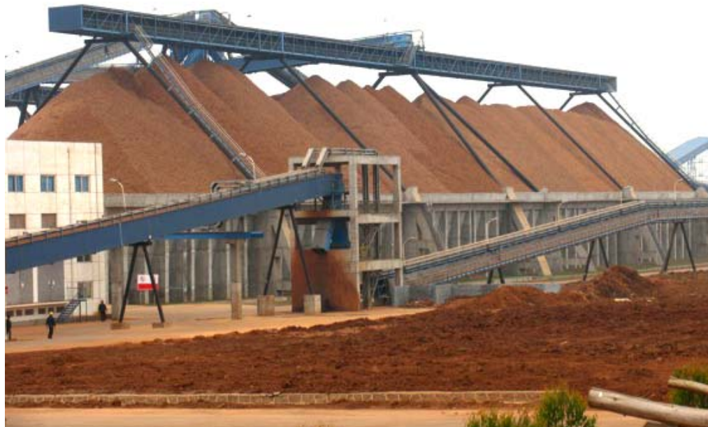
Eucalyptus chips are stored in two open chip piles, each with a volume of 150,000 loose-m 3 .
