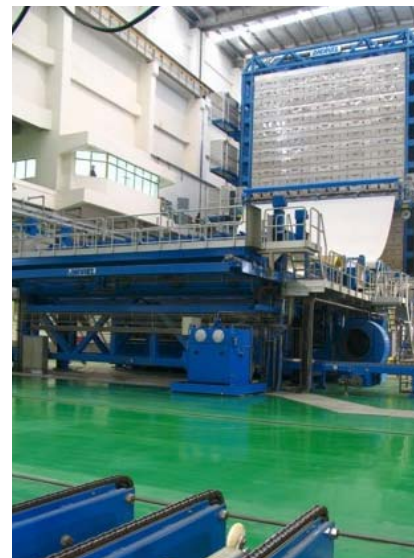
The Fläkt ™ dryer uses heated air to dry and support the pulp web. With the exception of the turning rolls at either end of the machine there are no moving mechanical parts inside the drying chamber.
