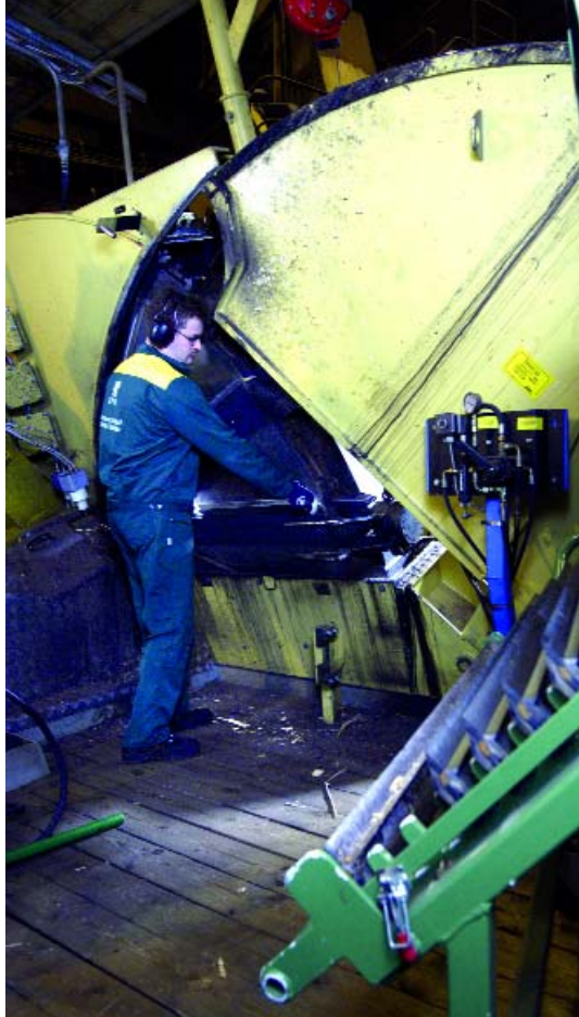
HQ-Plus™ makes routine knife changes at Wisaforest an easy, safe, and quick operation – for the best possible chipper availability.
