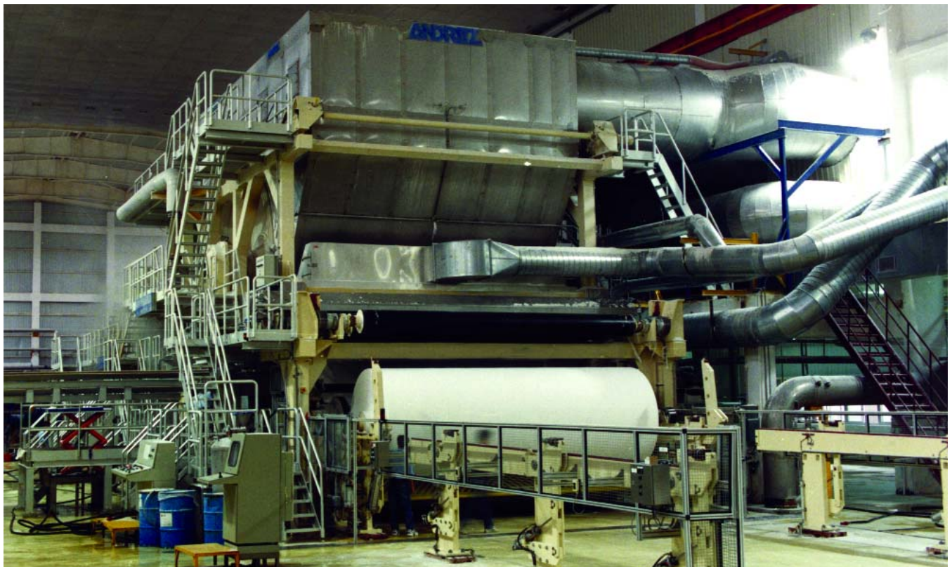
TM2 is one of the two identical CrescentFormer tissue machines at Gold Hong Ye. Both machines have a trim width of 5.6 meters and run at the highest average speeds in the world.
