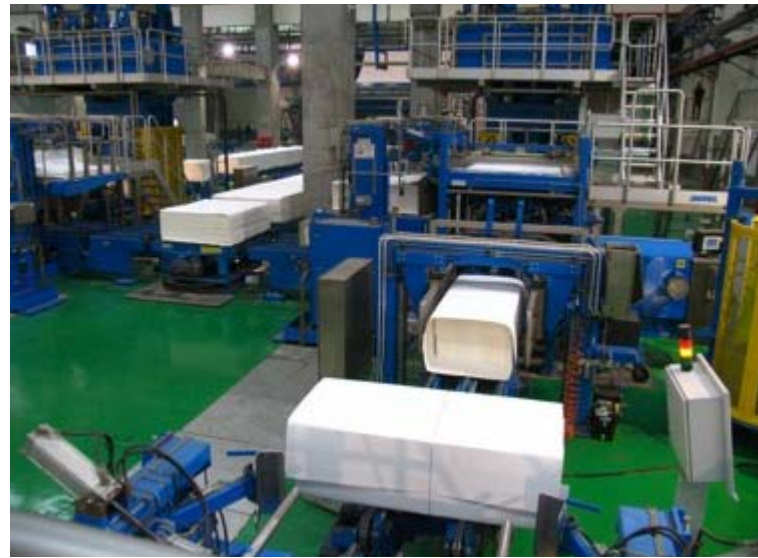
Pulp bales are pressed, wrapped, stacked four high, and tied together in two-ton units in the bale finishing line.
