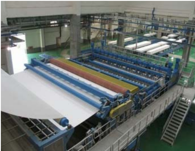
The world's largest cutter/layboy receives the pulp web from the dryer as the web is slit and cut into bale or wrapper-sized sheets.
