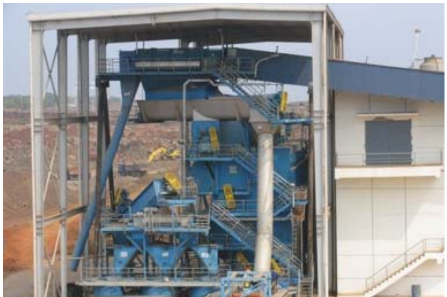
The JetScreen™ is new Andritz technology which uses air to separate the chip fractions. The JetScreen™ at Jiang Lin is the world's largest.
