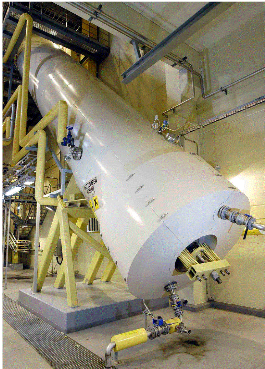
M&D Impregnator from the new Sawdust Cooking Line at Wisaforest, Pietarsaari. Start-up was summer of 2004.
