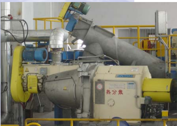
CompaDis™ disperser on the new DIP line.
