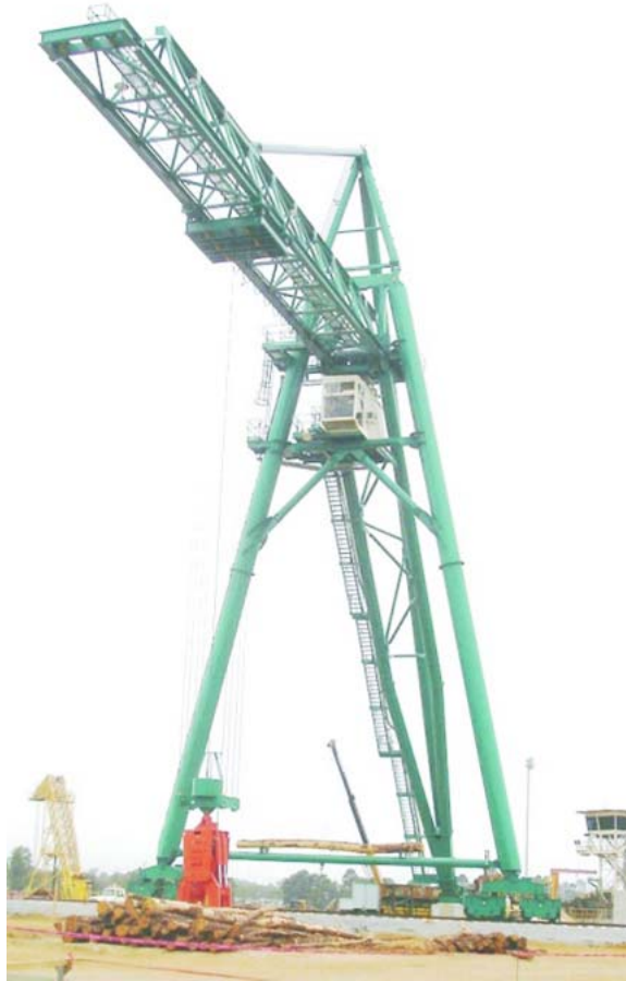
First 180 ft. radius circular crane started-up in October 2004 at Weyerhaeuser, Oglethorpe, GA, USA
