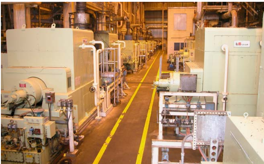
The conventional TMP plant at Calhoun produces about 1100 adt/d of pulp using Andritz (Sprout-Bauer) double-disc refiners. The plant was installed in 1979.
